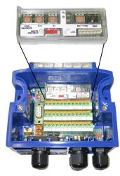
Figure 10 - BM100 Accessory Mounting
