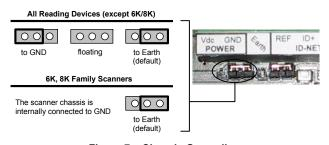
Figure 7 - Chassis Grounding
